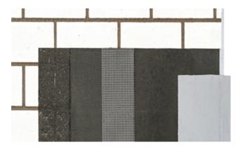
Superfleece embedded in KÖSTER MS-Flexfolie before the coat dries out. Apply the second coat, to cover the KÖSTER Superfleece. Make sure there is no air entrapped.
